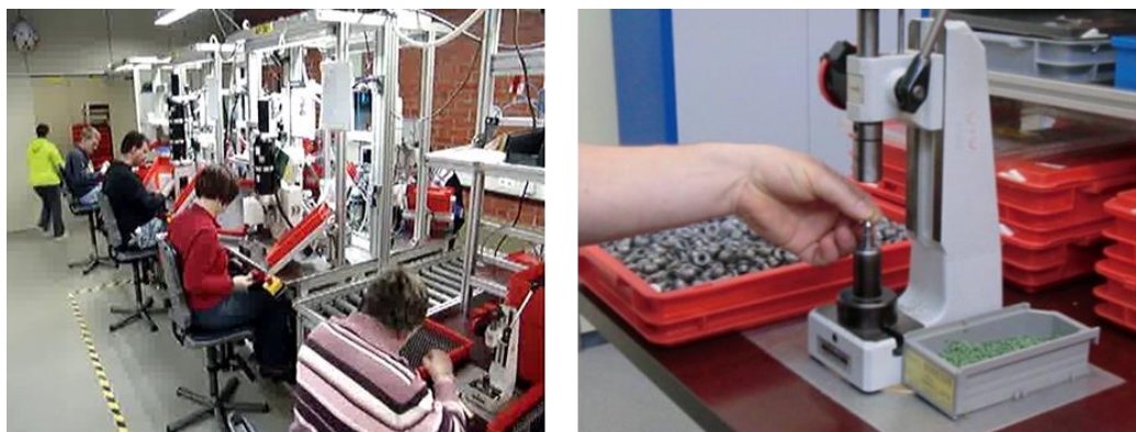
Figure 2: Manual assembly workplaces at the workshops for adapted work: Production line (left) and single assembly workplace (right). Source: Westpfalz-Werkstätten im Gemeinschaftswerk Pfalz.
