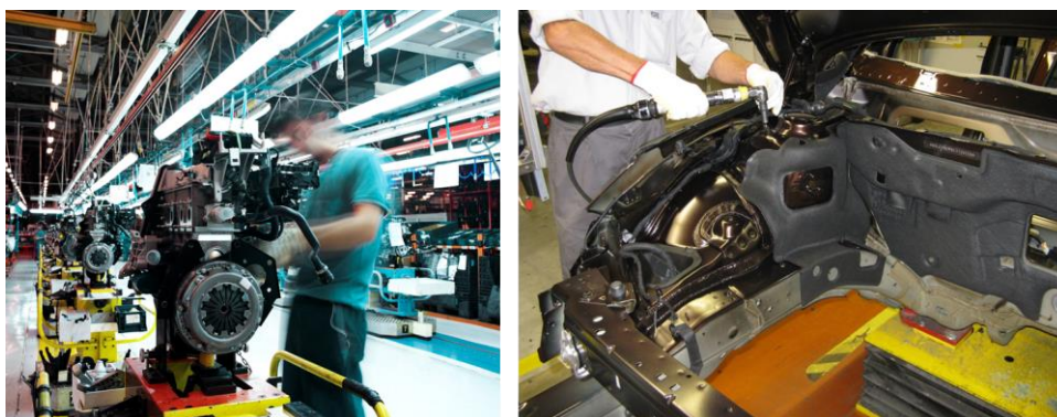
Figure 1: Manual assembly workplaces in automotive manufacturing: Production line for assembly of car engines (left) and work station for assembly at the car shell (right). Source: Adam Opel AG.
