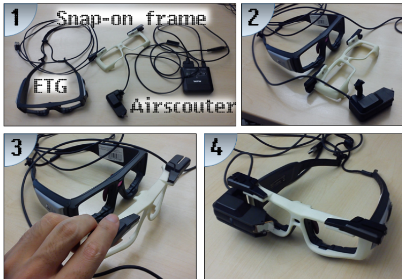
Figure 3.9: Assembling own eye trackable see-through display. 1) The ETG and the AirScouter. I printed a snap-on frame for fixing these two devices. 2) and 3) The ETG and the AirScouter is combined with the snap-on frame. 4) A complete eye trackable see-through wearable display. The position of the AirScouter could also be switched to left-eye.
