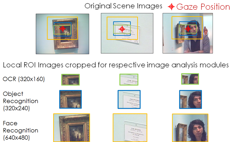
Figure 7.6: Local ROI image cropping. The size of a local image is determined by each image analysis module. The cropped image is used to recognize the visual content the user is fixating at in both AIA and CIA. The face detection would fail if the size is too small (in 320x160 or 320x240).
