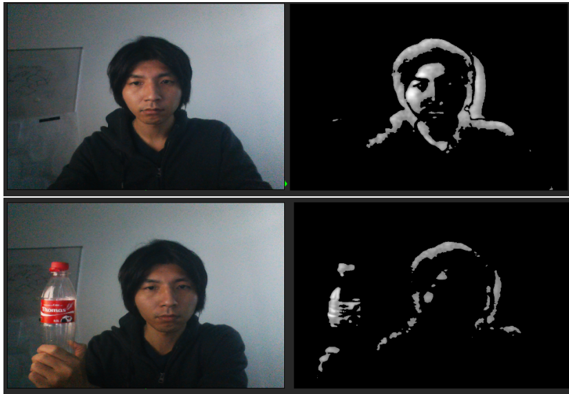
Figure 2.2: Examples of a saliency map. In the top image, the facial area is more salient than the other image region, whereas the label of a bottle is more salient than the facial area in the bottom image. We can clearly see the salient regions would draw human attention.
