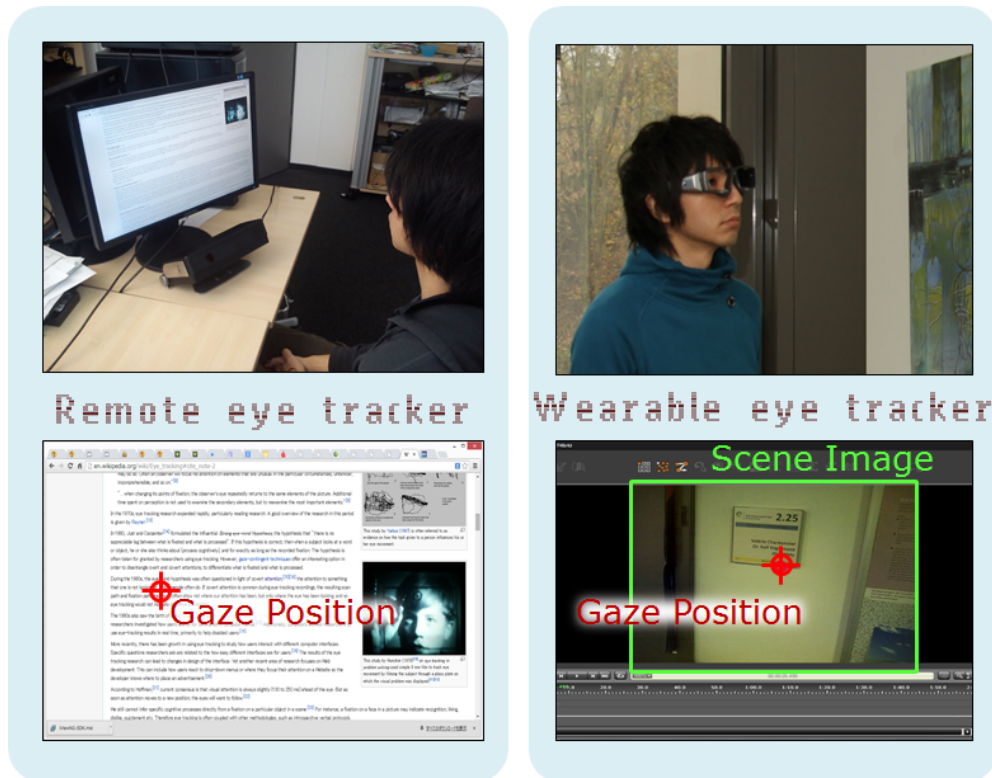
Figure 3.3: Remote eye tracker (left) and wearable eye tracker (right). A remote eye tracker is usually mounted on a desk and captures eye gaze on a computer screen. On the other hand, a wearable eye tracker captures a gaze focal point in a natural scene.
