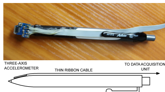
Figure 11.5: The accelerometer is mounted close to the tip of the pen
