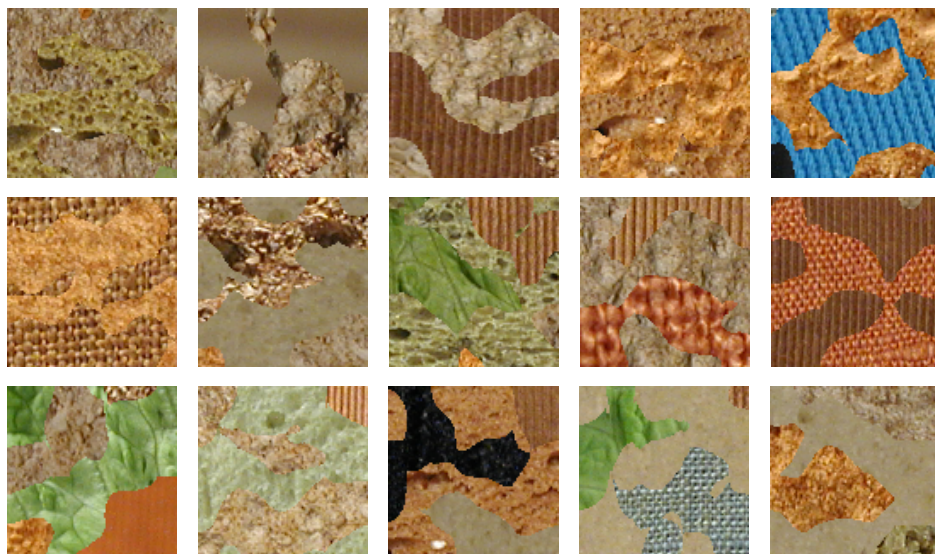
Figure 6.2: Blob-Mosaics texture segmentation database. The procedure of creating blob-mosaics image is as follows: 1) Gaussian filtering is applied on a randomly initialized image ( 100 \times 100 pixels with normal distributed values [0-1]). 2) Thresholding is performed for binarization (Median is selected as a threshold value). Randomly shaped regions are generated in this step. 3) Texture images from the KTH-TIPS2-a dataset [KTH] are randomly assigned to the regions. Note that, the dataset KTH-TIPS2-a itself includes material textures with various conditions (different scales, illumination directions, and poses). Thus, the final blob-mosaics images include random shapes in different positions, as well as textures under various transformations and conditions.
