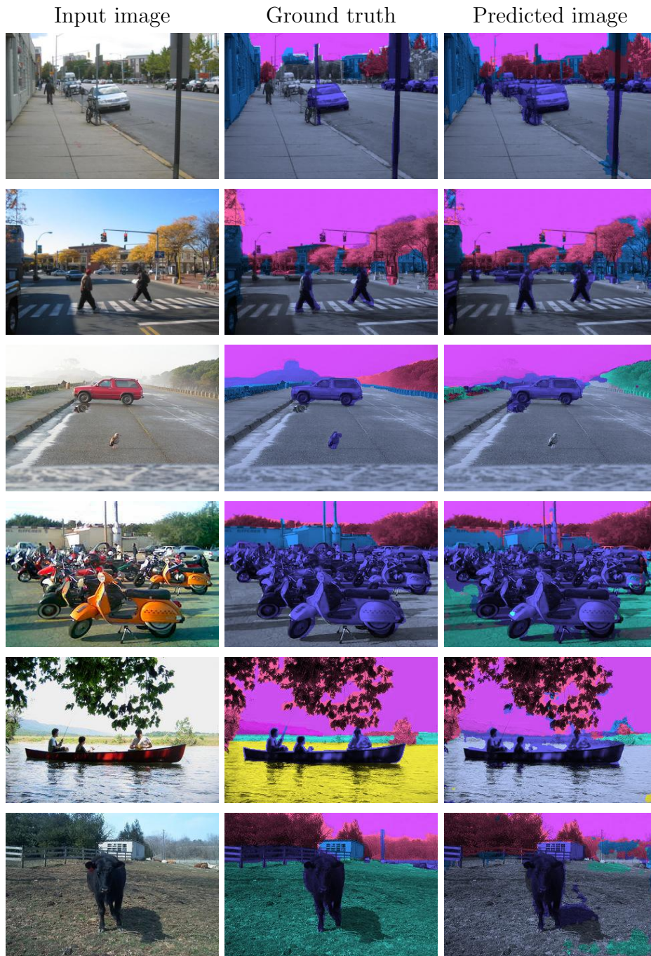
Figure 6.9: Selected mislabeled examples from LSTM networks. The first and second errors are mainly from mislabeling in the GT: human mistake — the car and human parts are labeled as “road” instead of its label “foreground” in the GT. The third misclassified regions are from very foggy forest. Furthermore, the reflection of a car wheel on the water is misclassified as a wheel (label “foreground”). These examples are understandable mistakes. The results show the difficulties of our dataset and the ambiguity of actual labels. The fourth to sixth examples show common mistakes of LSTM networks — the well-segmented regions are mislabeled. First row: road (gt) to grass (predicted); Second row: water (gt) to road (predicted); Third row: grass (gt) to road (predicted)
