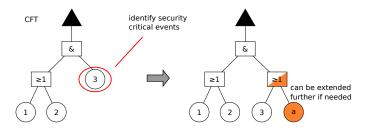
Fig. 1. Extension of a CFT.
