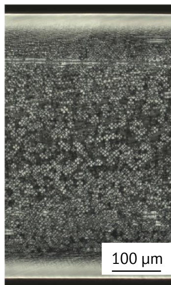
Figure 2.6: Skin-Core morphology of polypropylene [97].
