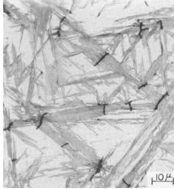
Figure 3.6: Micrograph of microcracks arising in plate-shaped martensite, Marder et al. [1970].
