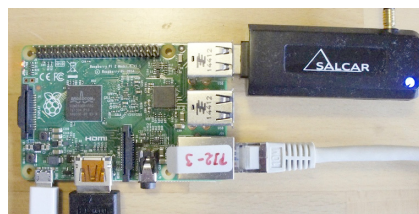
Fig. 1. A simple SDR receiver: Raspberry Pi with DVB RTL stick for low bandwidth processing
