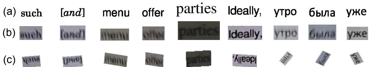
Figure 9.10: Word sample from an automatically generated dataset. (a) Ground truth image, (b) Normalized camera-captured image (c) camera-captured image with distortions
