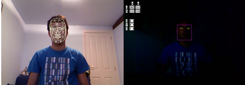
Figure 6.9: Kinect Face Tracking - Face and eye tracking based on Kinect sensor, left to right, CANDIDE-3 face model in Kinect Face Tracking Demo [FaceTracking], face and eye tracking under poor illumination condition [Gua12].
