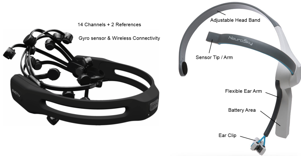
Figure 4.9: Brain-computer interface - Emotiv EPOC (left) [EPOC] and NeuroSky MindWave (right) [MindWave].
