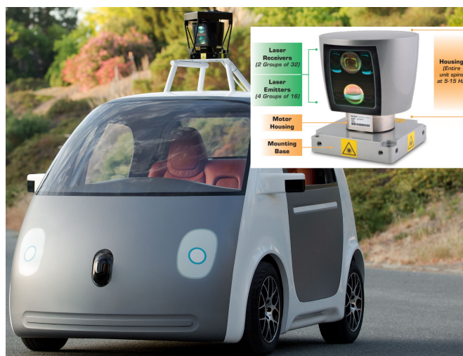
Figure 3.9: Google self-driving car prototype with Velodyne HDL-64E LIDAR sensor - Velodyne 64-beam LIDAR sensor is mounted on top of a Google driverless car collecting 3D information of car's surrounding environment [Google, Velodyne].
