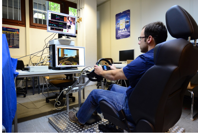
Figure 7.1: DeCaDrive demonstrator - The simulated driving environment of DeCaDrive (the final version).
