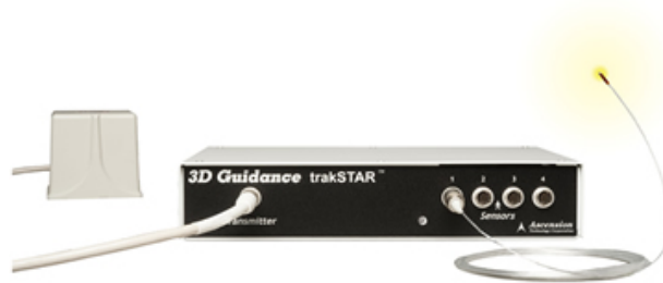
Figure 3.7: Ascension Trakstar System with transmitter and receiver. The search coil is directly connected to the processing unit.
