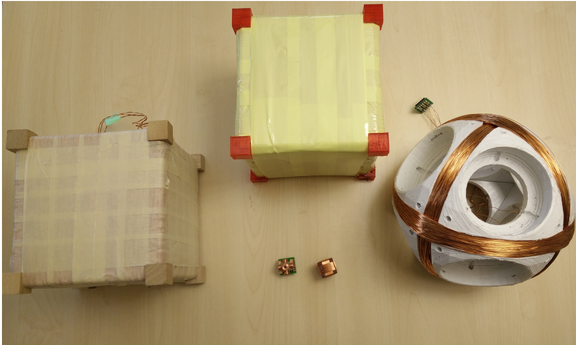
Figure 4.4: Different transmitter and receiver coil architectures left and center: cube shaped transmitter coils with three transmitter axes, right: circular transmitter coil with three transmitter axes and reduced crosstalk. Center front: 3D receiver coil with six conical axes, two coils are differentially amplified and sensed.
