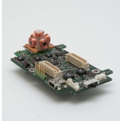
Figure 4.8: Receiver module of the magnetic field localization system. The three axes receiver coil measures the magnetic flux at the current location of the receiver.
