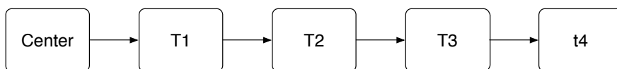
Figure 6.3: Deformed tree to estimate the timing offset introduced by using a hierarchical synchronization approach. The nodes t_i synchronize their clocks with t_{i-1} , t_1 with t_{Center} .
