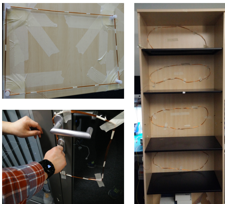
Figure 4.29: Upper left picture: Transmitter coil attached and coiling frame to easily create a coil. Lower left picture: transmitter coil attached to metal door, right picture: Rack with four transmitter coils, the current of each coil has been tuned so that the magnetic fields do not influence each other.
