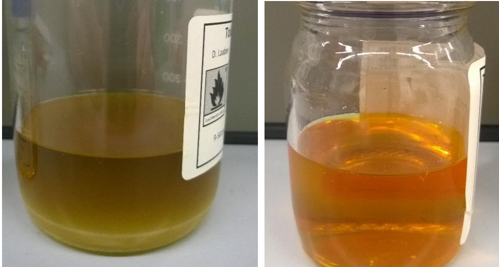
Figure 54: Colour change of the solvents: toluene - left, tetrahydrofuran - right
