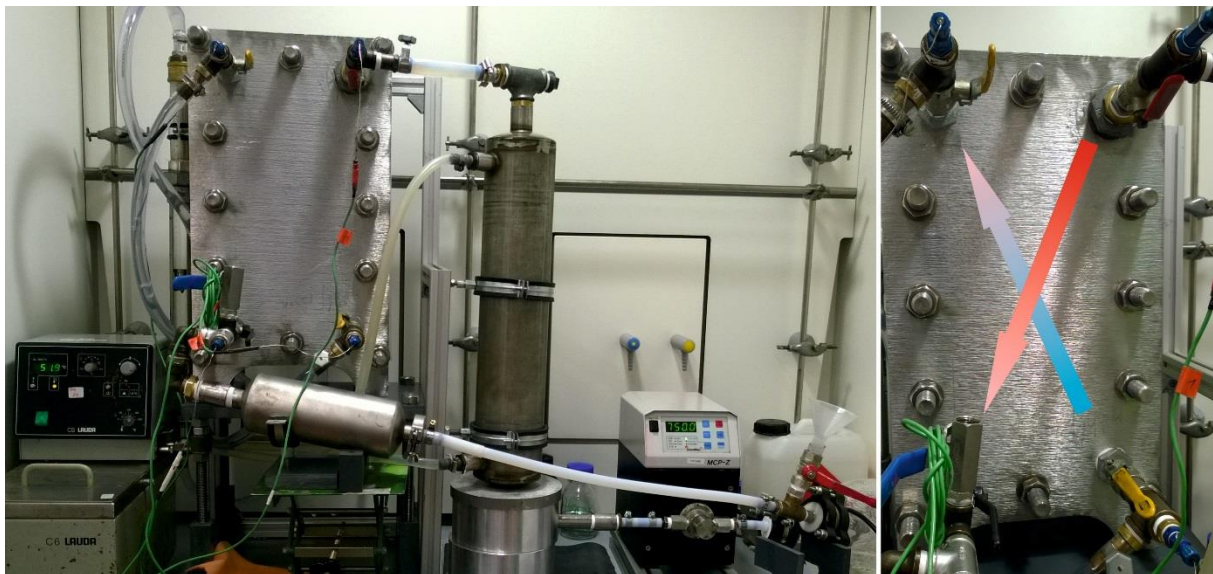
Figure 41: Heat transfer test rig with the large demonstrator mounted on it
