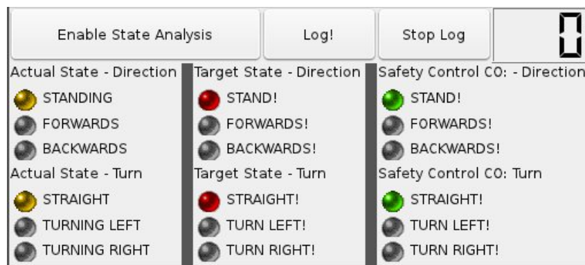
Figure 4.22: Example for dynamic data representation during test runs of complex systems in a frame of the MCAGUI [Gänßinger 11]
