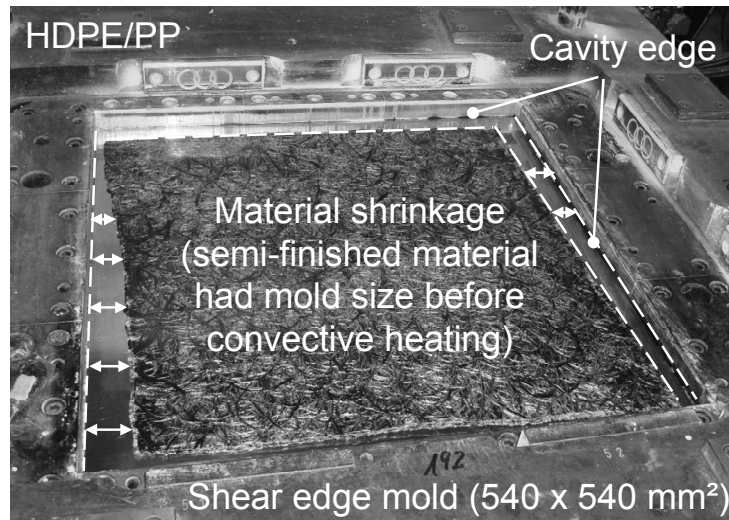
Figure 6.19: Visual shrinkage of HDPE/PP sheets after convective heating
