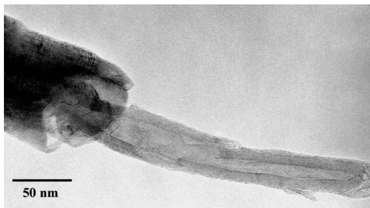
Figure 1.8: Evidence of nanotube broken by the sword-in-sheath fracture mechanism in MWNT/PS composite film [127].
