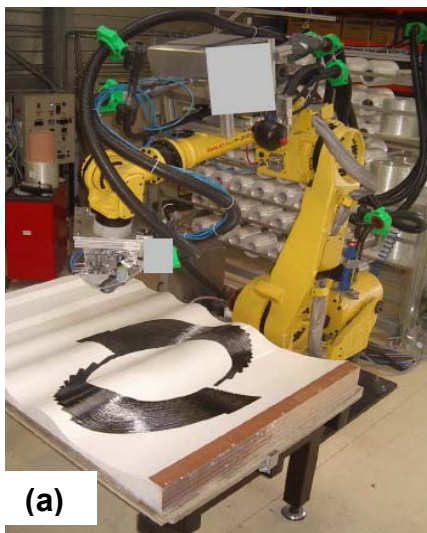
Figure 2.1: Automatic tape placement head attached to robot arm / gantry (a) for thermoset material [5] (b) thermoplastic material [6].
