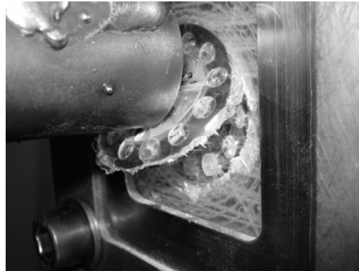
Figure 3.53: The characteristic failure mode of the unstitched inserts Type A (Type of specimen: Type 1)
