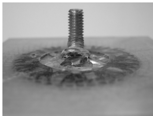
Figure 3.54: Characteristic failure mode of the carbon thread stitched inserts Type A (clamping distance: s = 6 mm) (Type of specimen: Type 10)
