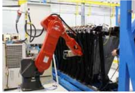
Figure 2: Induction weld robot and weld jig for Gulfstream G650 rudder torsion box [33,34]
