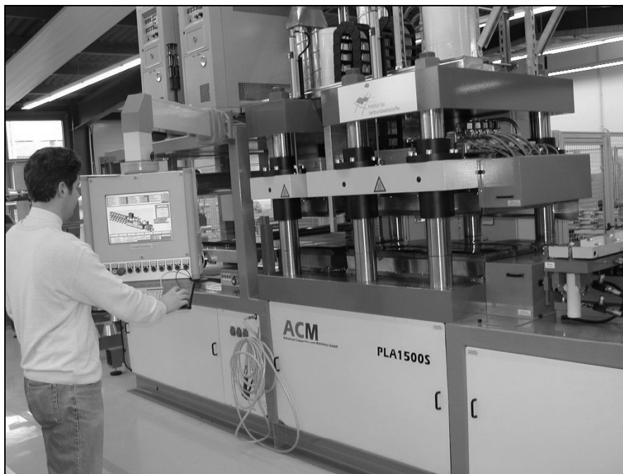
Figure 1.2: Continuous compression molding press at the IVW
