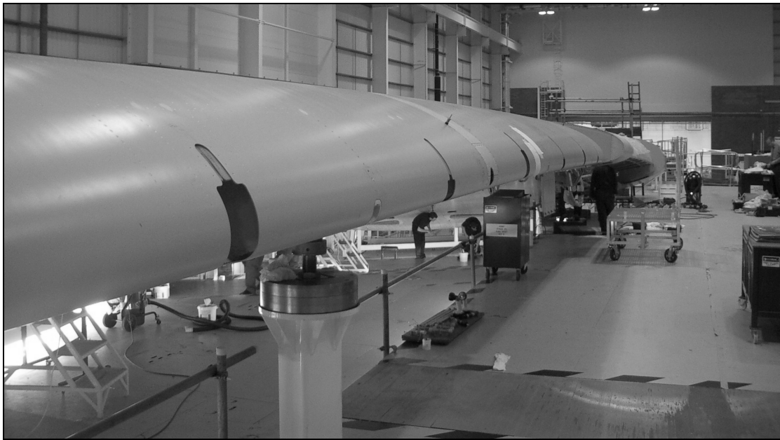
Figure 1.6: J-Nose mounted on a wing for an Airbus A380 (© Airbus United Kingdom)
