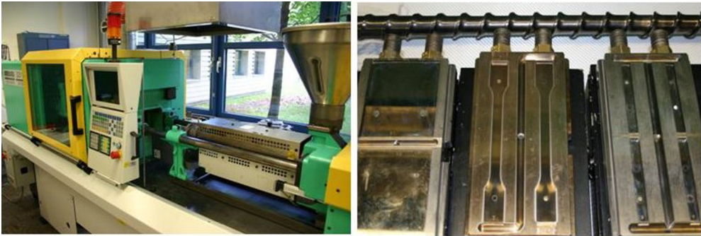
Figure 3.6: Arburg injection moulding machine and used mold templates.
