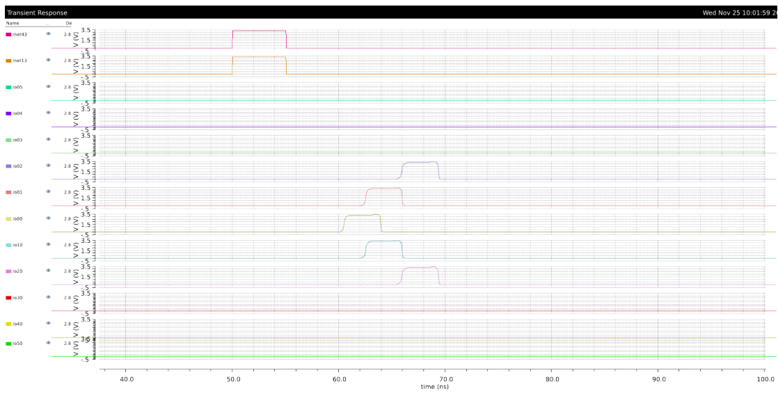
FIGURE 6.26: Post-layout Simulation (showing coincidence detection with minimum Gaussian kernel width. It is the counterpart of the Figure 6.6)
