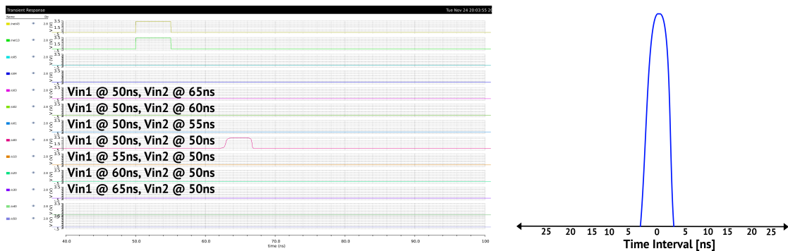
FIGURE 6.4: Simulation showing Coincidence Detection (with minimum Gaussian kernel width) (left), A Sketch of the corresponding Gaussian Kernel (right)
