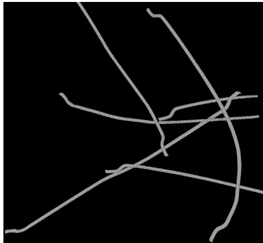
Figure 6.12 – One of the fiber clusters from CT image of steel fiber reinforced concrete (image size: 791 \times 232 \times 943 voxels).
