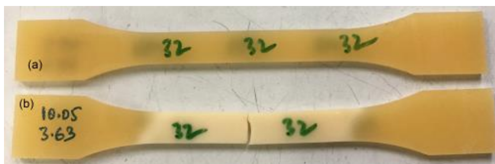
Figure 69: Tensile sample (a) before the test and sample (b) after the test showing the stress-whitening due to void formation during tensile tests.
