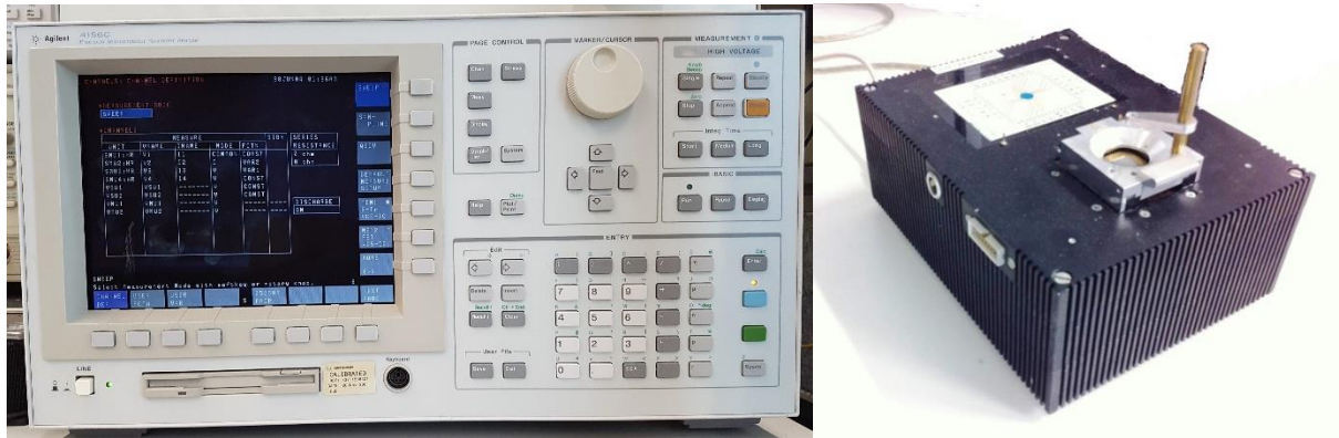
Figure 5-4 Available measurement setups: Agilent 4156C Precision Semiconductor Parameter Analyzer ( http://www.keysight.com ) (left), TTF box (right)
