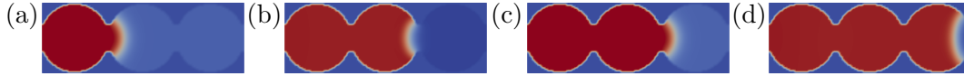
Figure 4.53: Lithium ion concentration for a cathode built of multiple spherical particles. (a)-(d) \text{SOC} \in \{0.45, 0.66, 0.76, 0.96\} .
