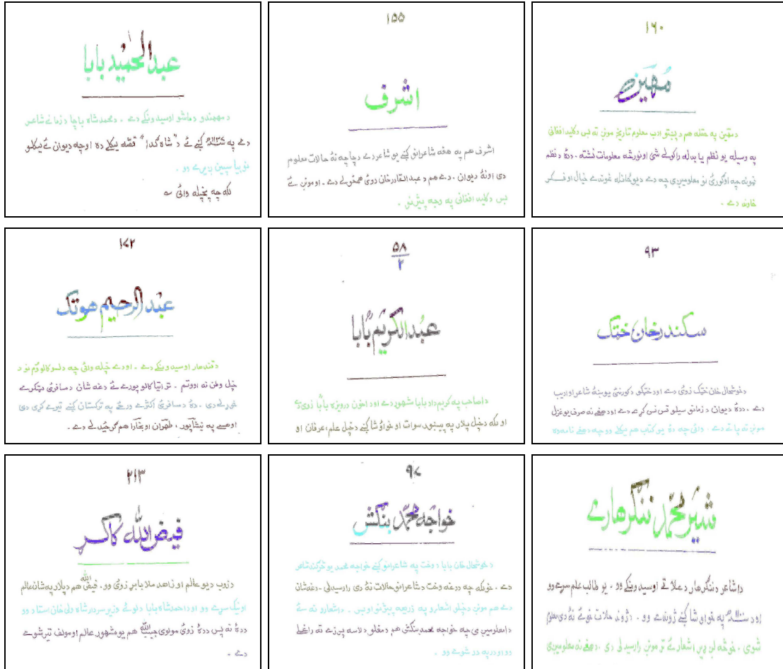
Figure 9.2: The segmentation results of Ryu’s method [RKC14] on Pashto text documents. The titles are split into two or three text-lines. In these cases, the tuning of the parameters \alpha and \beta does not work.
