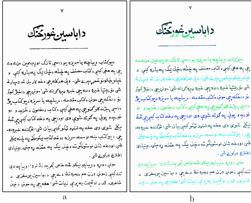
Figure 9.1: Input binary image (a) and the segmentation result (b) from the method [RKC14] (with default parameters). Note that, the page number is merged with a title, and the title is split into two lines.
