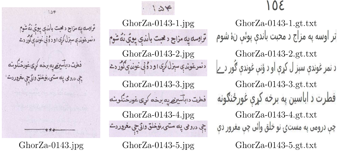
Figure 7.3: An input image with its file name below it (left), their corresponding extracted text lines along with their file names (middle) and ground truth and their naming convention for files (right). Image source: [AAR + 16]
