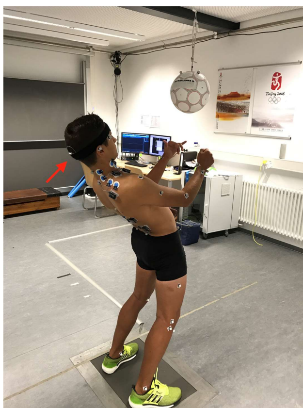
Figure 1. Test design for the variant from a standing position. The red arrow points to the 3D accelerometer in the occipital area.
