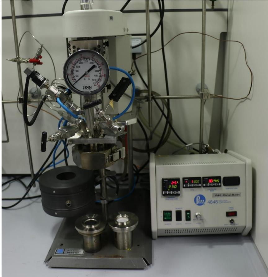
Abbildung 14. High pressure autoclave from Parr. Right side: control unit with values for stirring, temperature and pressure. Left side: autoclave with heating mantle and two vessels (one with Teflon<sup>®</sup> inlet).
