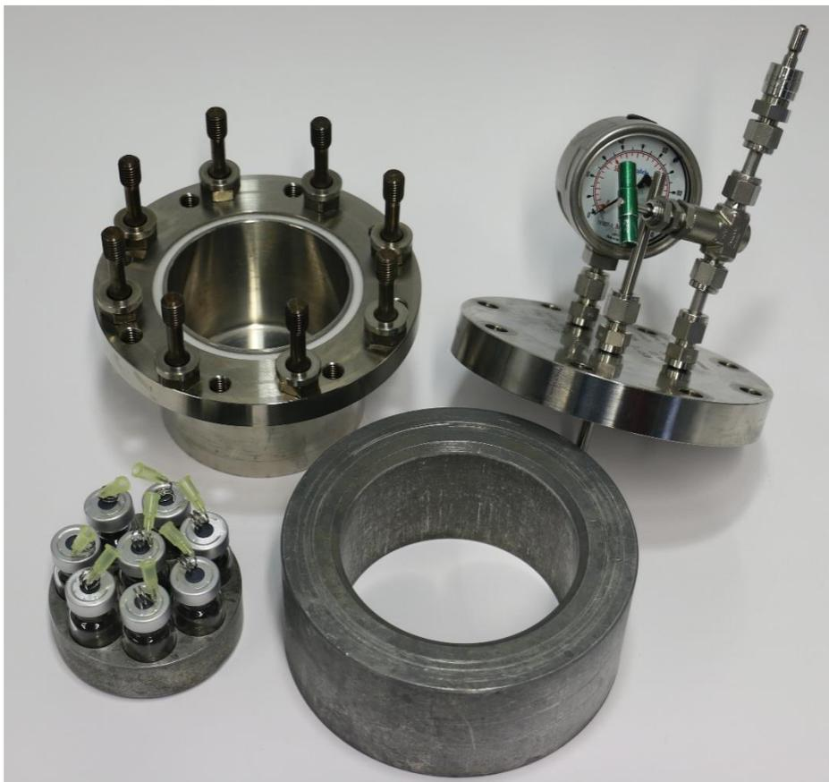
*Abbildung 13. Standard autoclave with inlet (filled with 8 reaction vials punctured by cannulas), cover, heating mantle and expansion screws.*
