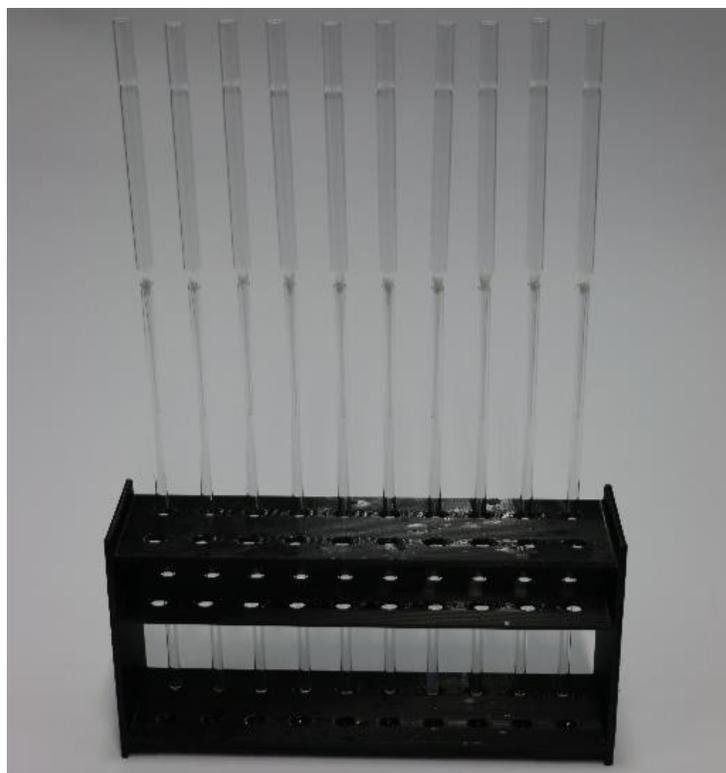
*Abbildung 16. Standard set-up for the NMR work-up of 10 parallel reaction mixtures with NMR tubes and glass pipettes as filters.*
