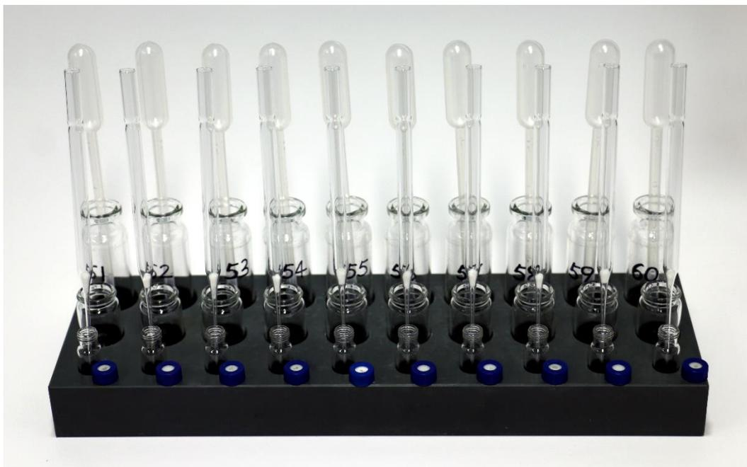
Abbildung 15. Standard set-up for the GC work-up procedure of 10 parallel reactions with reaction vials (back), work-up vials (middle), GC vials (front), plastic pipettes (back) and glass pipettes as filters (front).
