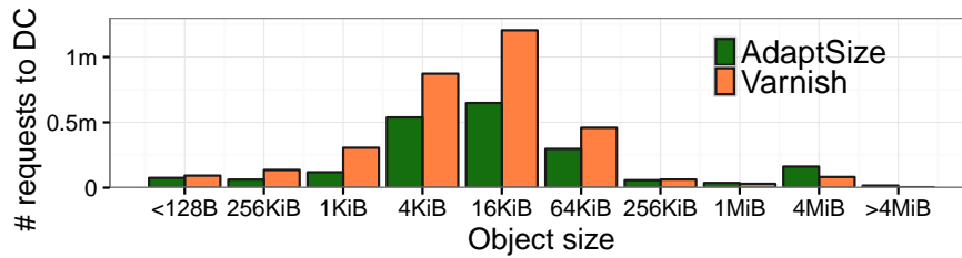
Figure 3.16: Comparison of the distribution of request sizes to the disk cache under a HOC running AdaptSize versus unmodified Varnish. All object sizes below 256 KiB are significantly less frequent under AdaptSize, whereas larger objects are slightly more frequent.
