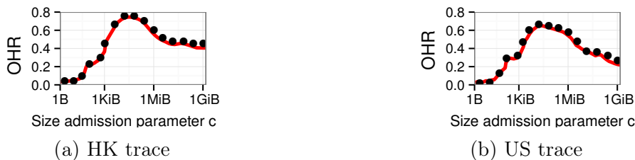
Figure 3.7: AdaptSize’s Markov model predicts the OHR sensitivity curve (red solid line). This is very accurate when compared to the actual OHR (black dots) that results when that threshold is chosen. Each experiment involves a portion of the production trace of length \Delta = 250K .
