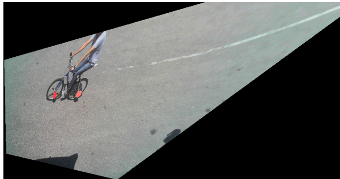
FIGURE B.2: Ground projected camera image. To be seen are the bright red markers attached to the wheels of the bicycle
