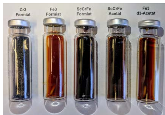
Figure 31 Picture of several metal carboxylate complexes after synthesis using the classical method.
