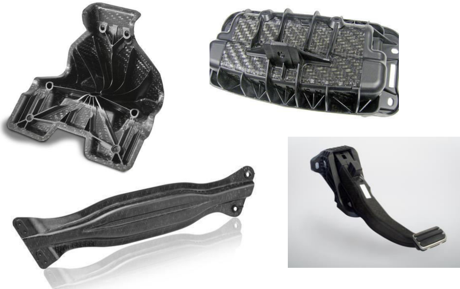
Figure 2.2: Hybrid-molded automotive components by the aid of local reinforcement with continuous fiber reinforced thermoplastic materials [18][19][20]
