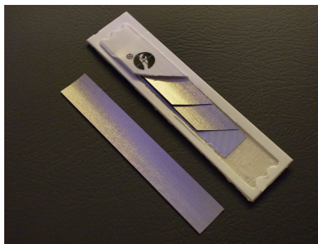
Figure 1.1: Cut-away view of a typical acousto-magnetic tag (distributed under a CC0 1.0 license).
