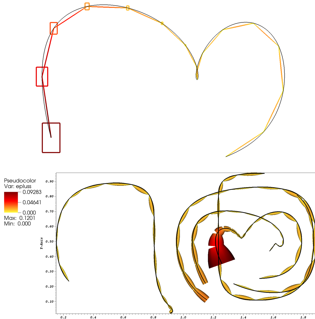
Figure 3.4: Double gyre. Top: A reconstructed path line is shown with the estimated global truncation error e from (3.19) represented by rectangles. Bottom: Five reconstructed path lines are represented as tubes with a radius equal to the absolute estimated error a from (3.22), which also determines the color. On both sides, the corresponding correct path lines are plotted in black.
