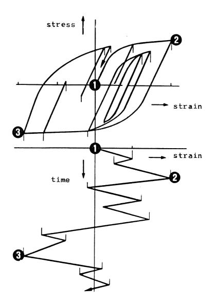
The counting result is stored in the so-called Rainflow matrix A and the Residuum R. The elements a of A are the number of closed hysterisis loops from level "i" to level "j". These loops are also called Rainflow cycles and may be defined as follows:
