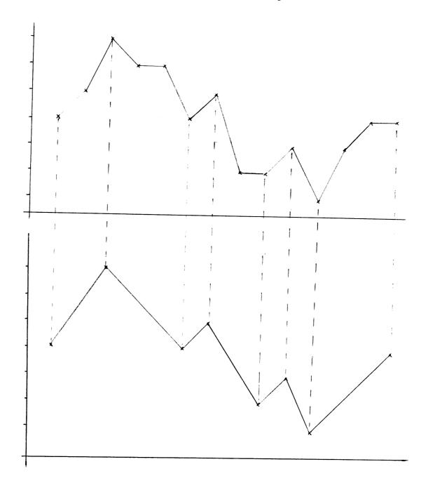
Fig. 1: Reduction of the load time function to a peak/trought sequence.
