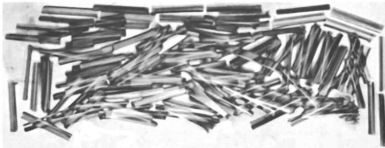
Figure 2.8: PP-LGF50, x-ray image of pellets with lead glass fiber fraction
