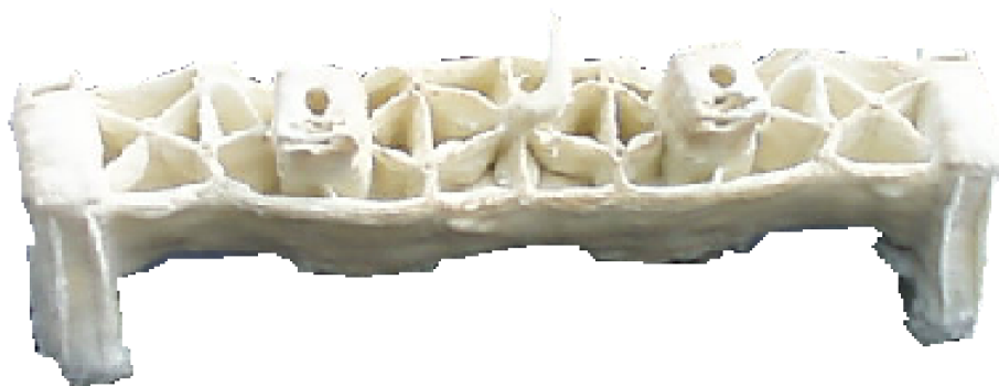
Figure 2.3: Fiber skeleton of passenger seat component
