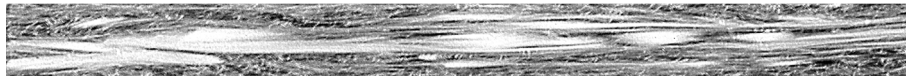
Figure 2.6: Microstructure of PP-LGF50, x-ray image of the cross-section parallel to the main direction of flow
