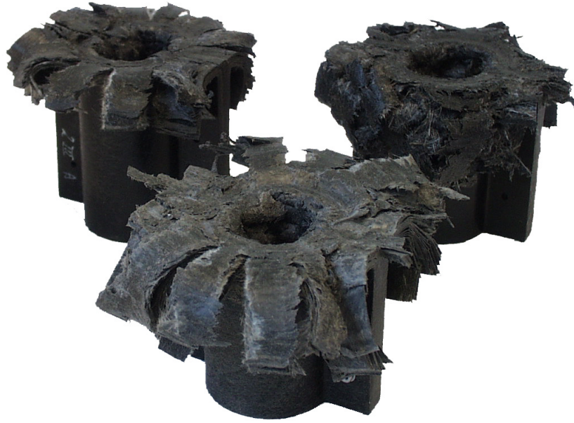
Figure 24: Crash elements of PP/GF30C (left), PP/GF30C_MF (front) and PP/GF30R (right)
