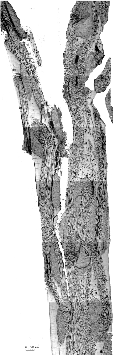
Figure 71: Micro-photograph of the crush zone of GF/PET(C)
