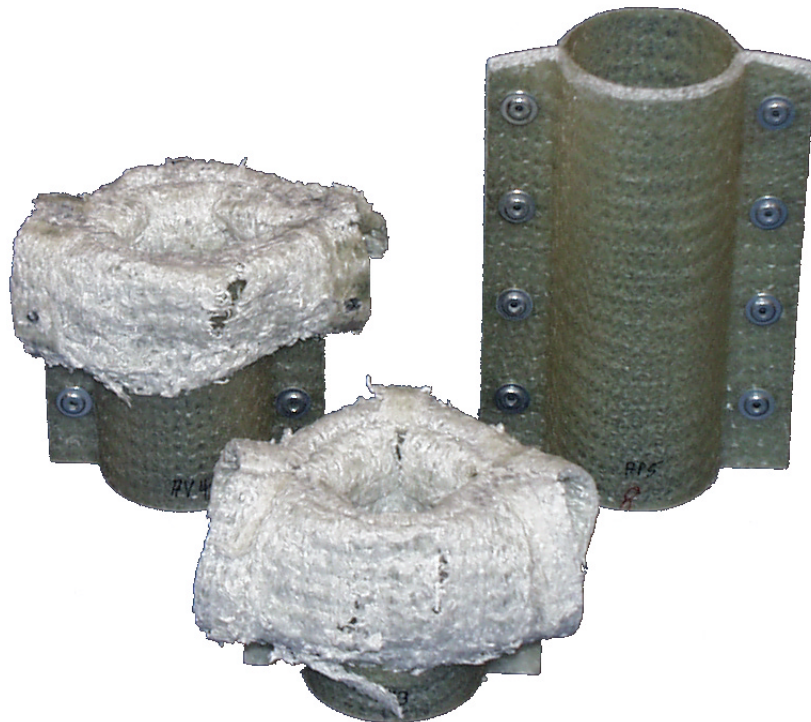
Figure 18: GF/PET(A) crash elements showing the macroscopic failure behaviour
