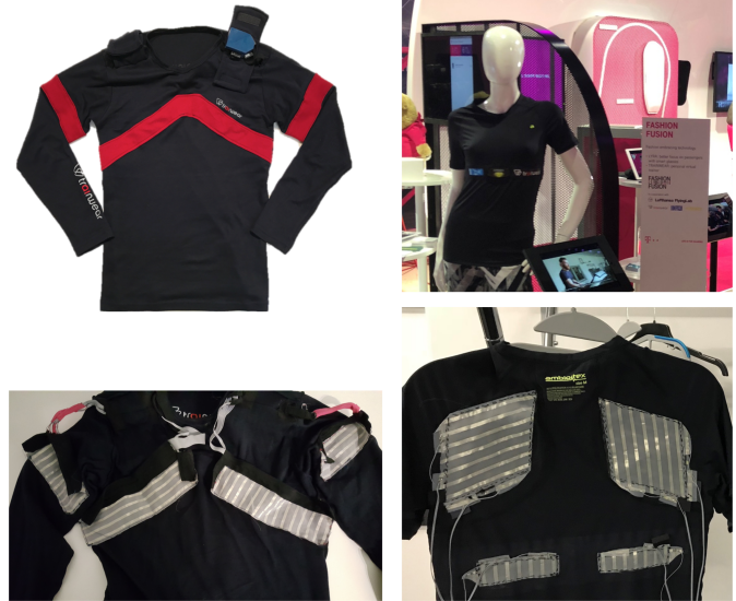
Fig. 61. TPM sensors can also be buried under a slim fit clothing without stretch band support for body motion monitoring.
