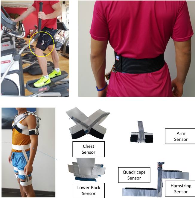
Fig. 60. TPM sensors can be integrated into stretch bands that targets different body part movements.
