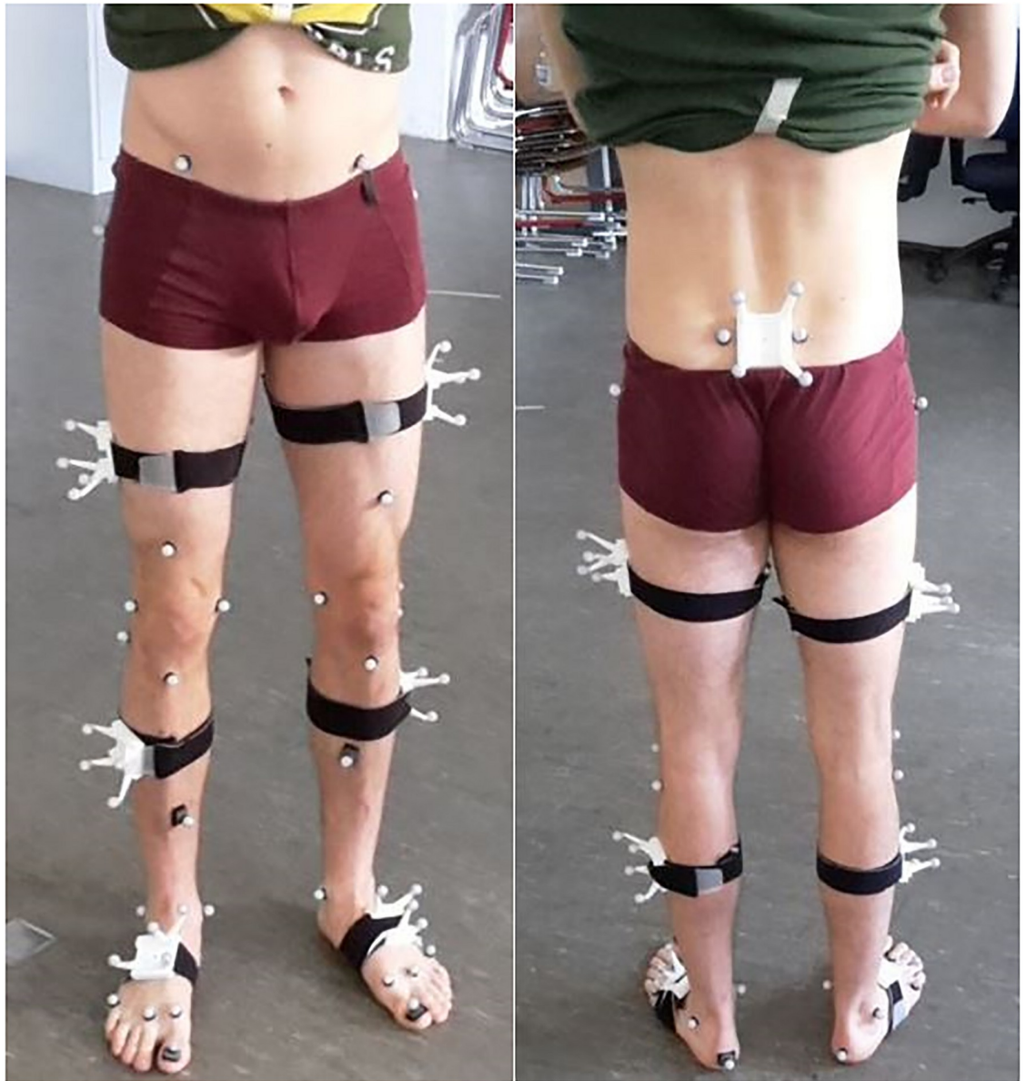
Fig 2. Marker protocol and IMU placement. Retroreflective markers attached to the anatomical landmarks and the RMC. IMU are not inserted in the RMC in this schematic picture.
