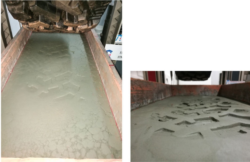
Figure 45: Quarry fines' footprint photographs.
