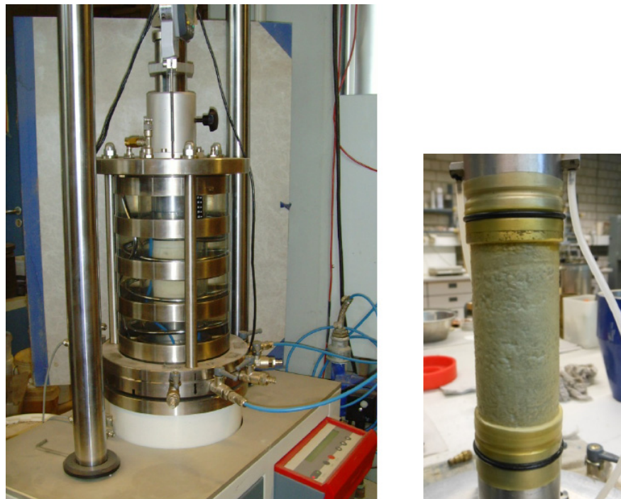
Figure 16: Triaxial test apparatus and soil sample.
