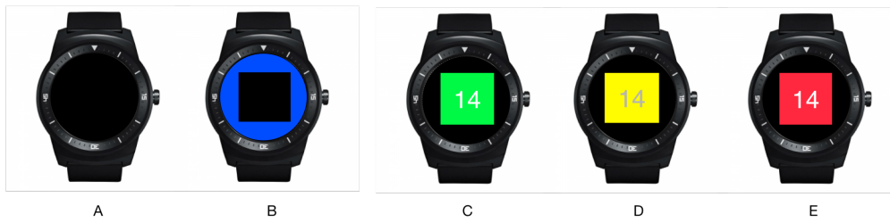
Figure 5.1: CPR smart-watch App: vibration and a blue/black (A, B) blinking with 110 cpm; color feedback about detected compression depth display center (green (C) - good, yellow (D) - beyond recommendation, red (E) - not sufficient)
