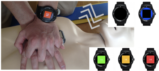
Figure 5.11: CPR Watch Assistant is providing frequency instructions and instant feedback on compression depth and speed while performing CPR!
