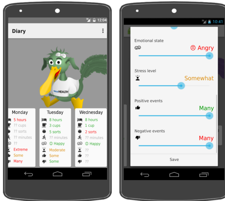
Figure 2: Screenshots of the MVP. Left: main screen with avatar and diary summary. Right: diary scales with color coded entries to provide feedback on the conformity of the user's behavior with the health recommendations.
