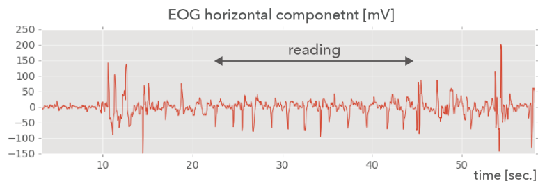
FIGURE 3.26: EOG sensor signal in one-minute recording including reading activity.
