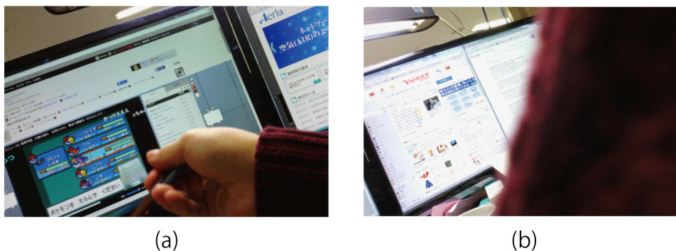
FIGURE 3.24: Samples of errors in natural reading detection. (a) false negative: a user is browsing web pages. (b) false positive: a user is watching a video.
