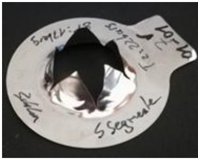
Figure 34: Open rupture disk device.
