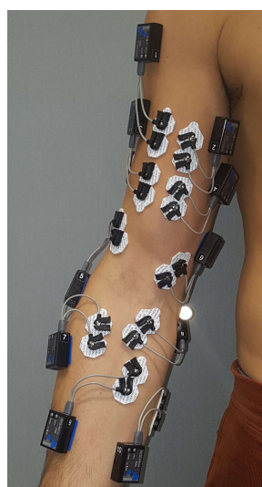
Figure 19: Placement of several wireless bipolar surface EMG electrodes on upper arm and forearm.
