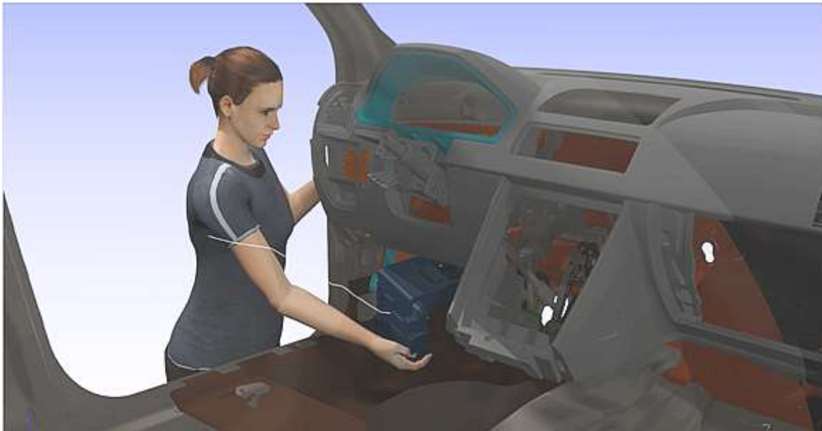
Figure 1: Assembly analysis using a digital human model. Source: IPS IMMA software.
