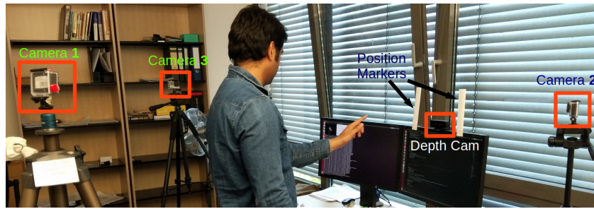
Figure 7.2.: Our setup for in-air signature acquisition. The depth camera is mounted on top of the screen. The position markers on both sides of the depth camera allow capturing of in-air signature within the field of view (FoV) of the camera. Three GoPro cameras are placed around a user to record the hand motion in 3D space from different view points. Camera 3 specifically records the depth variation.
