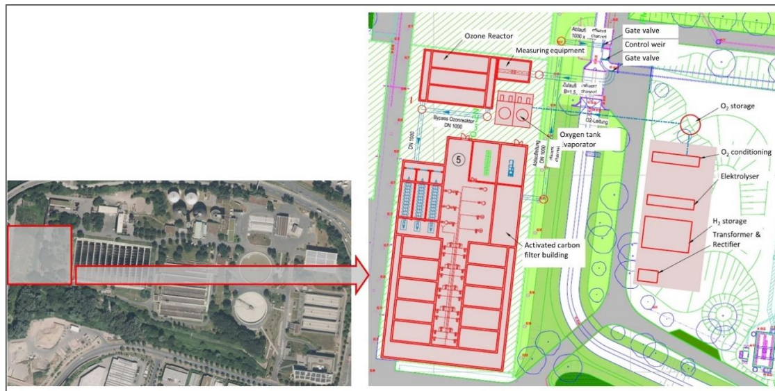
Figure 5. Aerial view of WWTP Mainz ( www.geoportal.rlp.de ; “Data license Germany—attribution—Version 2.0” referring to the license text available at www.govdata.de/dl-de/by-2-0 ; left side) and extract of a side plan with the new system components (right side) [41].
