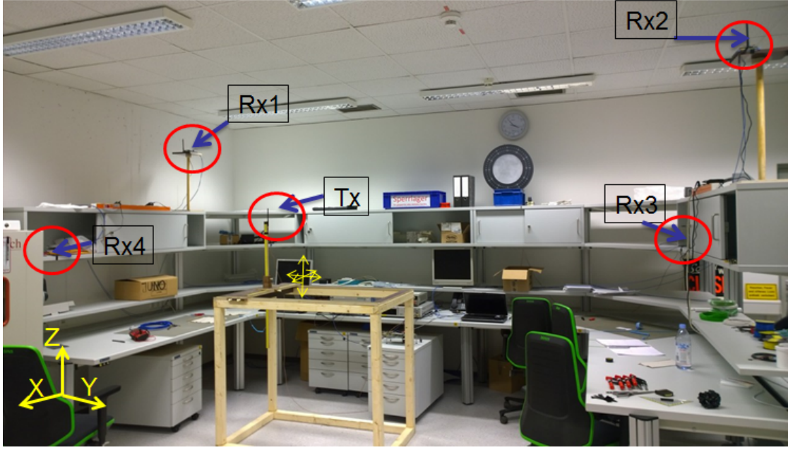
Figure 4.16: 3D test in a Lab environment, 4 receivers and 1 target transmitter.
