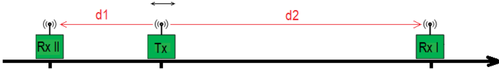
Figure 4.8: The range difference from the transmitter to the pairwise receivers is to be determined.
