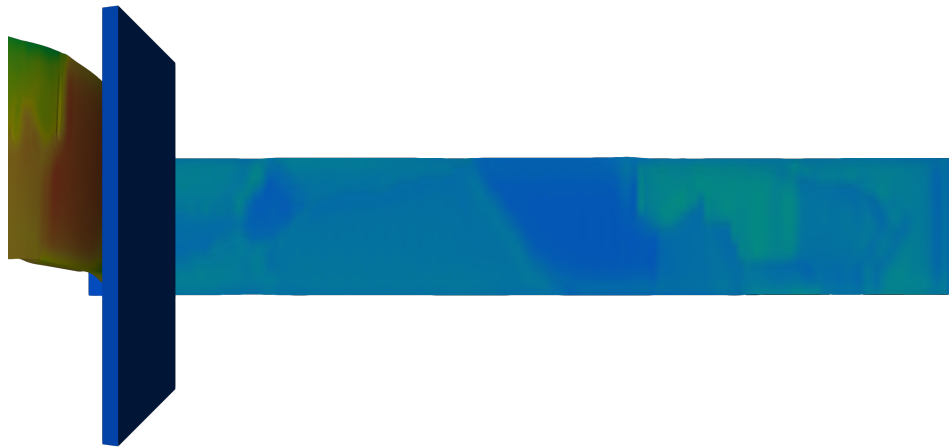
(a) Main and \langle c+a \rangle slip systems with \tau_0^1 = 145 MPa.
