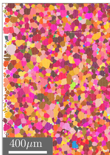
FIGURE 1.1: EBSD picture of the micro structure of a cp-titanium sample (Bischof et al. (2018)).
