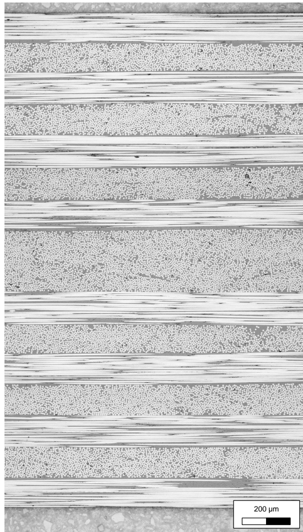
Figure B.2: Exemplary cross-section of (0^\circ/90^\circ)_{4S} laminate. The cut was realized along the 0^\circ direction.
